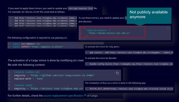
Screenshots from Siemens developer portal describing how to configure the mirrors for various tools and environments.
